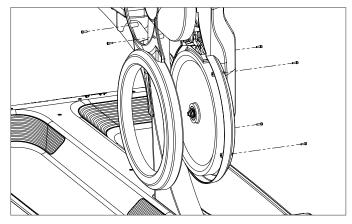
b. Check brake pad setting by first turning the resistance knob toward the "-" sign as far as it will go (minimum braking effect). The brake pad should have approximately a credit card thickness between it and the flywheel and the brake pad should feel slightly loose around its pivot. If adjustment is required see **TROUBLESHOOTING GUIDE** (see page 13).
