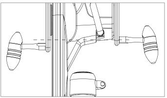
Turn the resistance knob toward the "+" sign until the crank arms do not fall by themselves back to the lowest rest position. Raise the crank arms so the crank handles are nearly level. Loosen (do not remove) the 5 socket head cap screws (B) on the RIGHT crank arm with a 4mm ALLEN KEY WRENCH. Adjust the position of screws within the slots until both crank handles are level and then tighten. Make sure all screws are tight, or the crank handle may slip out of synchronization again.
