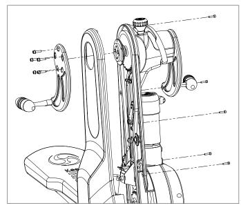
Check cable and cable sheath (A) for excessive wear (replace if necessary). If the lever still exhibits excessive play, tighten the adjustment screw (B) clockwise until play is removed. Be careful not to over tighten the adjustment screw as the pivoting mechanism may not fully engage and could lead to machine failure or injury.
