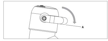
Remove rotation lever and cap by removing 2 socket head cap screws with a 4mm ALLEN KEY WRENCH. Loosen (do not remove) upper set screw (B) on upright frame with a 3mm ALLEN KEY WRENCH.
