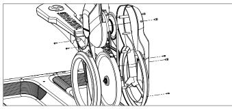
If the chain is rubbing on the inside covers or exhibits too much play around the sprockets the chain should be replaced by a service technician.
