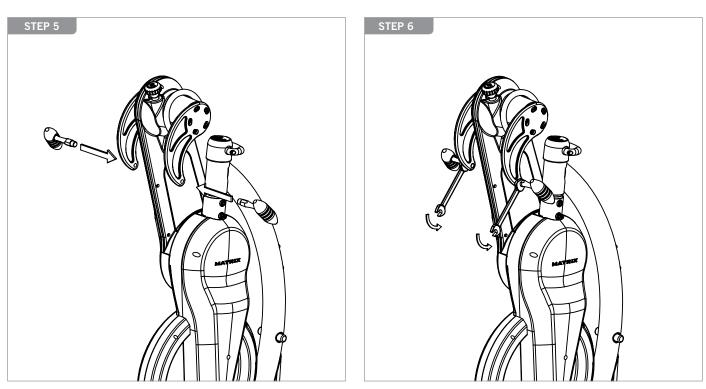
Attach LEFT HANDLE to LEFT CRANK ARM and RIGHT HANDLE to RIGHT CRANK ARM. Please note the LEFT HANDLE has a left hand thread.
