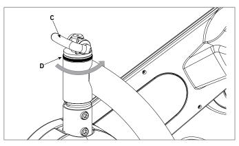
To complete adjustment tighten upper set screw and replace rotation lever and cap.
