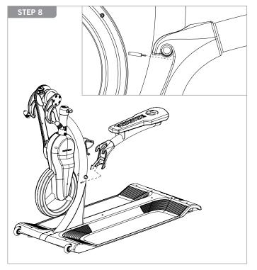
Attach SEAT to UPRIGHT FRAME by securely placing SEAT HOOKS around PROTRUDING PIN.\*\*\*
