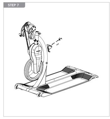
Attach WATER BOTTLE CAGE to CENTER UPRIGHT FRAME with 4mm ALLEN KEY WRENCH using item 4-SOCKET HEAD CAP SCREWS.
