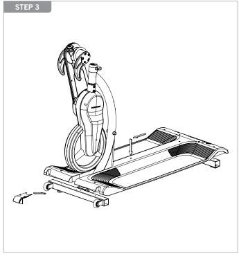
Place SMALL BASEPLATE FRONT COVER and LARGE MAIN BASE PLATE on metal frame.
