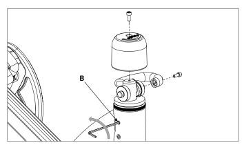
Replace rotation lever, and release rotation cam mechanism (C). Rotate cam plate (D) counterclockwise 1/8 of a turn and then engage rotation cam mechanism. Repeat until the upper drive arm is held rigidly without play. The rotation lever should require a firm force to fully engage. If the rotation lever is too difficult to engage, reverse the previous steps.
