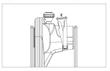
Remove the RIGHT crank arm by removing 5 socket head cap screws with a 4mm ALLEN KEY WRENCH then remove the upper outside plastic cover by removing 5 socket head cap screws with a 3mm ALLEN KEY WRENCH.
