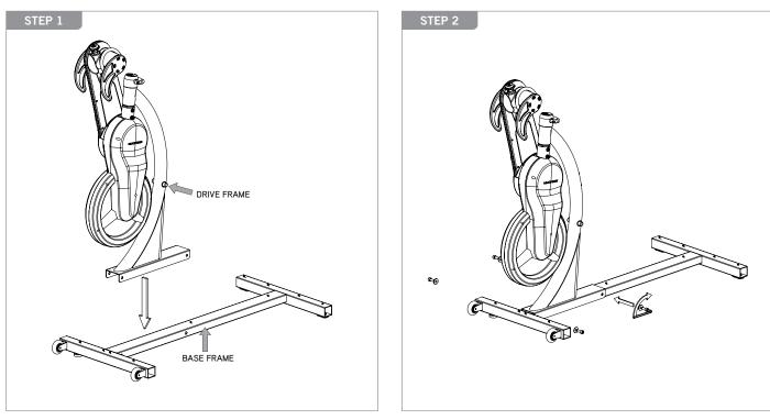
Place DRIVE FRAME on BASE FRAME so the bolt holes line up.
