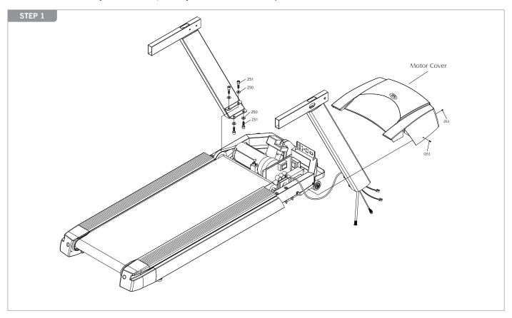
Unscrew the screw (Q53) on each side, and keep the screws. Remove the motor cover.
