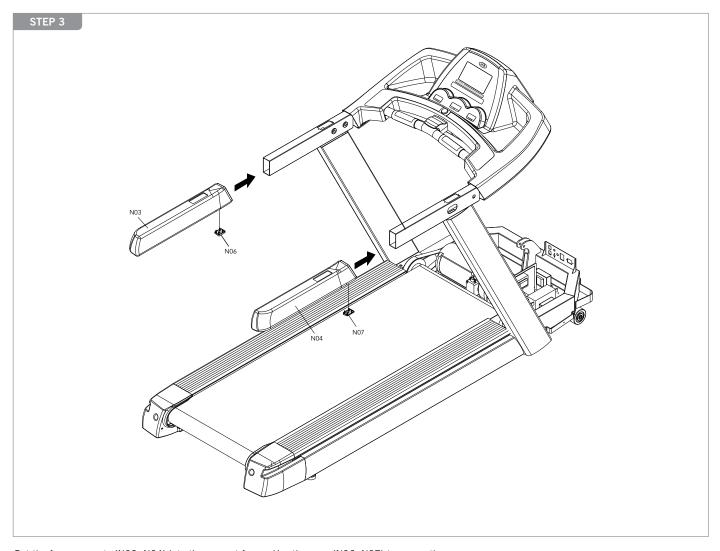
Put the foam armrests (NO3, NO4) into the armrest frame. Use the caps (NO6, NO7) to secure them. Note: The caps separate into right and left, make sure these caps are in the correct position.
