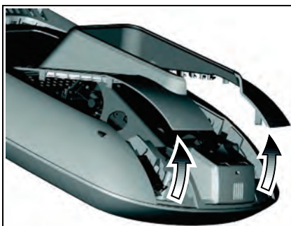
Figure 22: Removing the access cover from the P80 console
